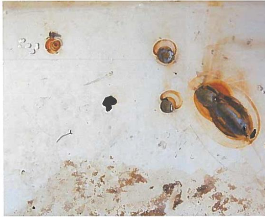
52. Metal loss in floor.
