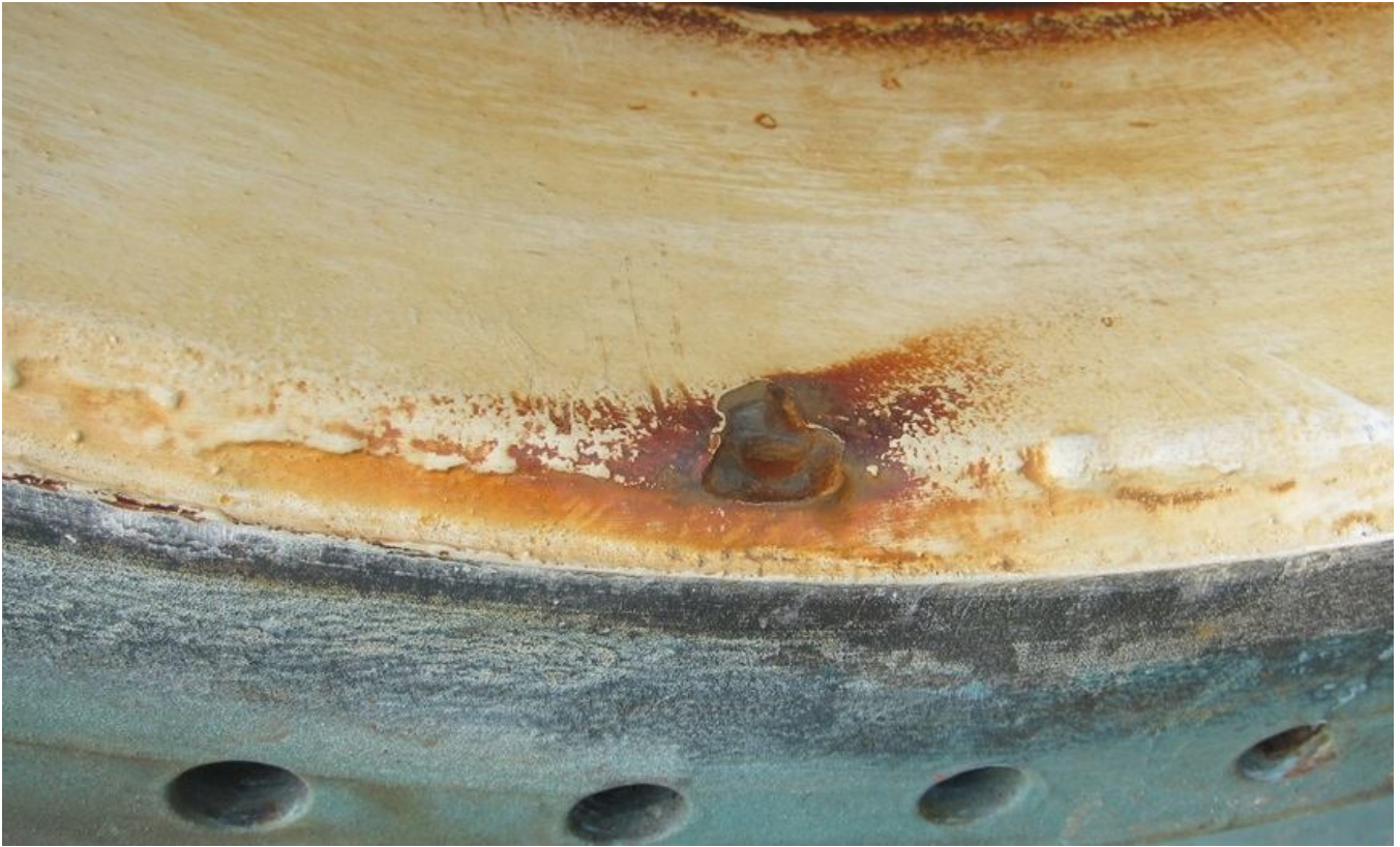
15. Corrosion and metal loss in shell manhole neck.
